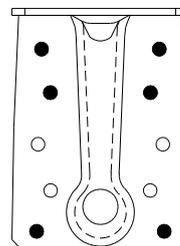
Beam to steel (6 mm S355) connection
