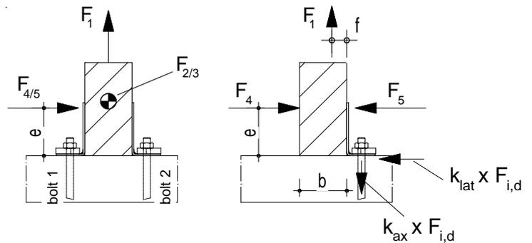
Each bolt shall have a capacity to sustain a lateral force of:  $\geq k_{\text{lat}} \times F_{i,d}$
