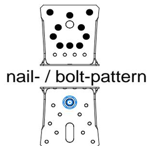
*Table D12-7 2 angle brackets ABR100, timber beam to 6 mm steel beam connection – connector nails + PAT pins*
