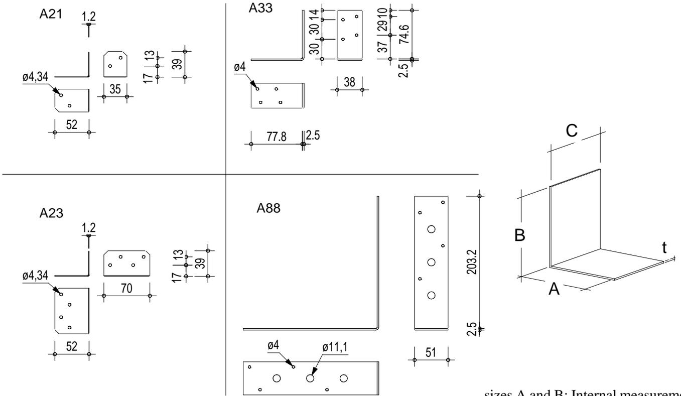
sizes A and B: Internal measurements
