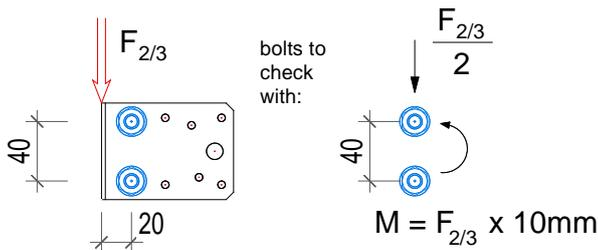
Table D2-5 1 Angle Brackets AB90, beam to rigid support connection
