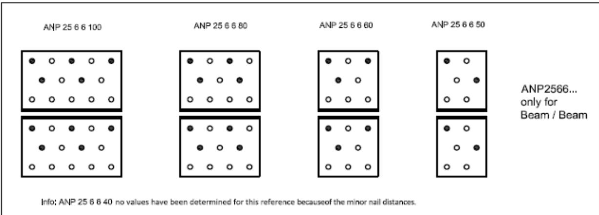
**Table D53-4: Characteristic capacity beam to beam (connection with two ANP)**
