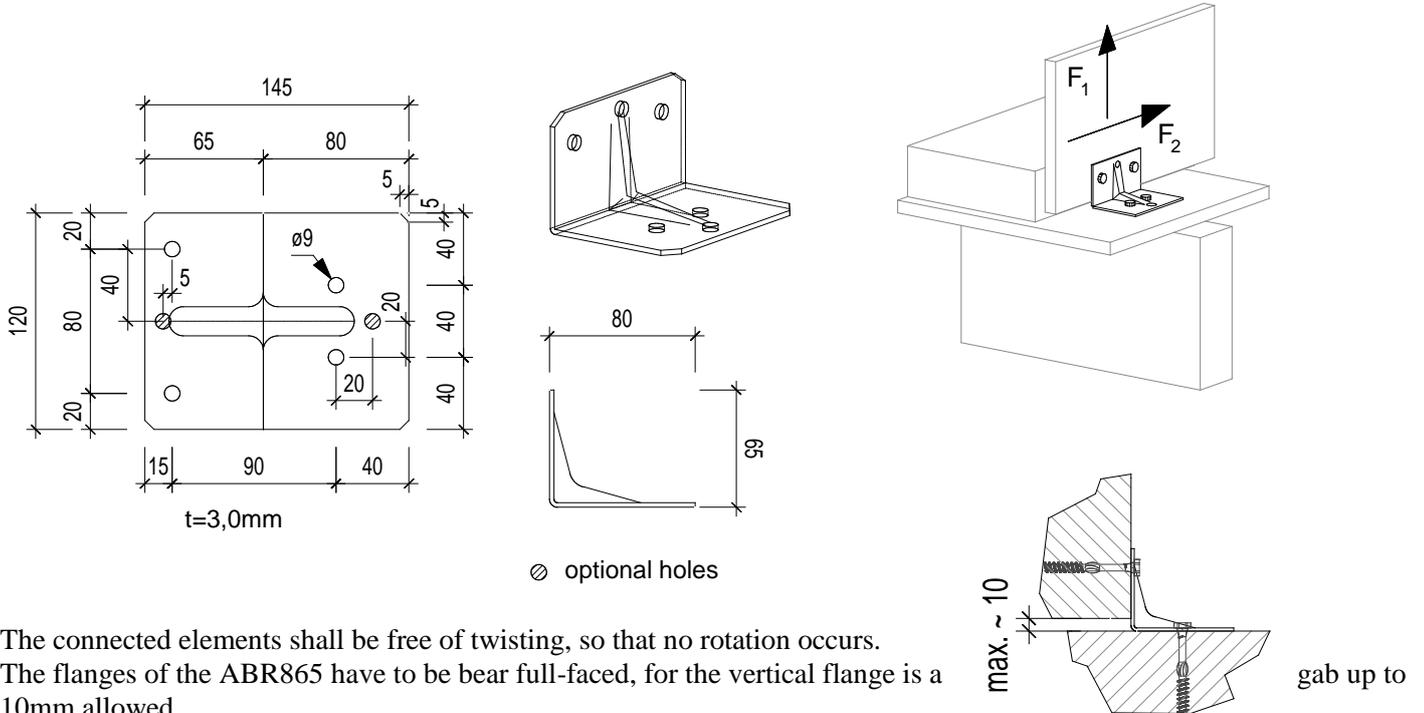
The connected elements shall be free of twisting, so that no rotation occurs. The flanges of the ABR865 have to bear full-faced, for the vertical flange is a 10mm allowed.
