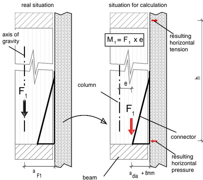
Generally the brackets shall be calculated with a lever arm of  $F_1$  of  $a_{F1} = ( a_{dia} + 8mm )$
