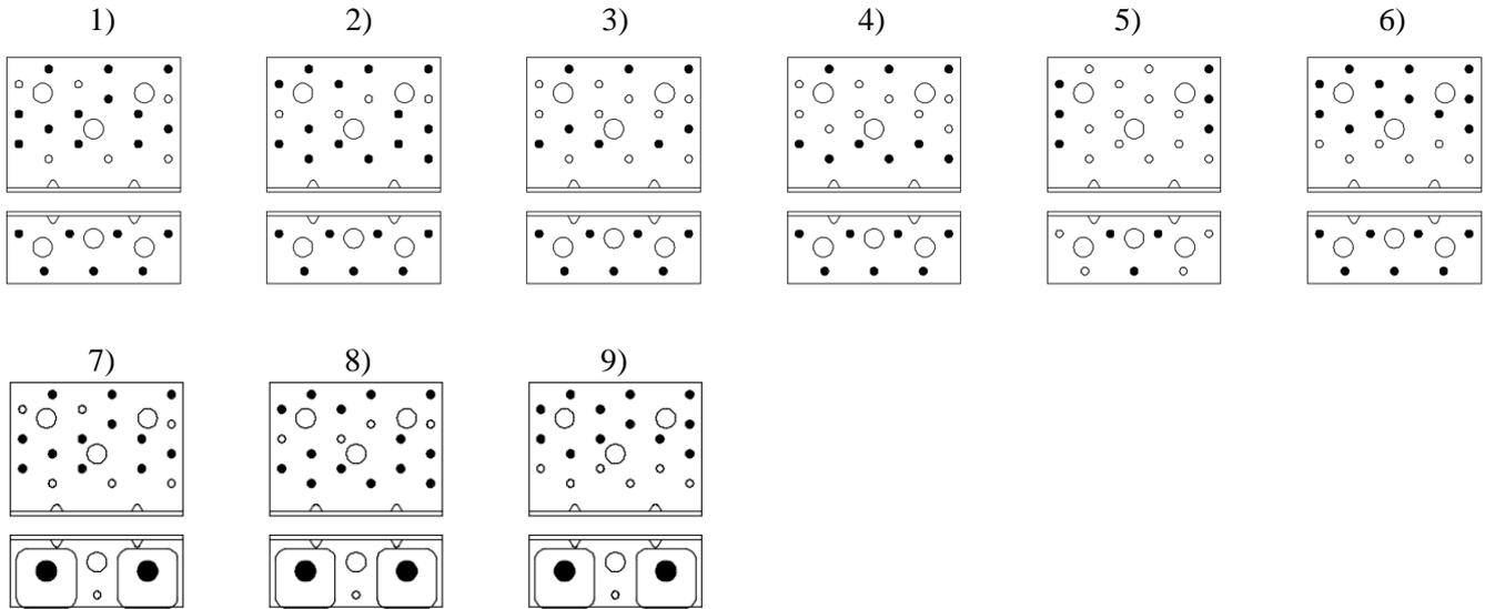
Square washer (US40/40/10G or US40/50/10G) can be replaced by standard washer of the bolts (bolt Ø12 – washer Ø24). In this case the value of  $k_{lat}$  and  $k_{ax}$  must be adapted (see tables below D17-4 and D17-5).
