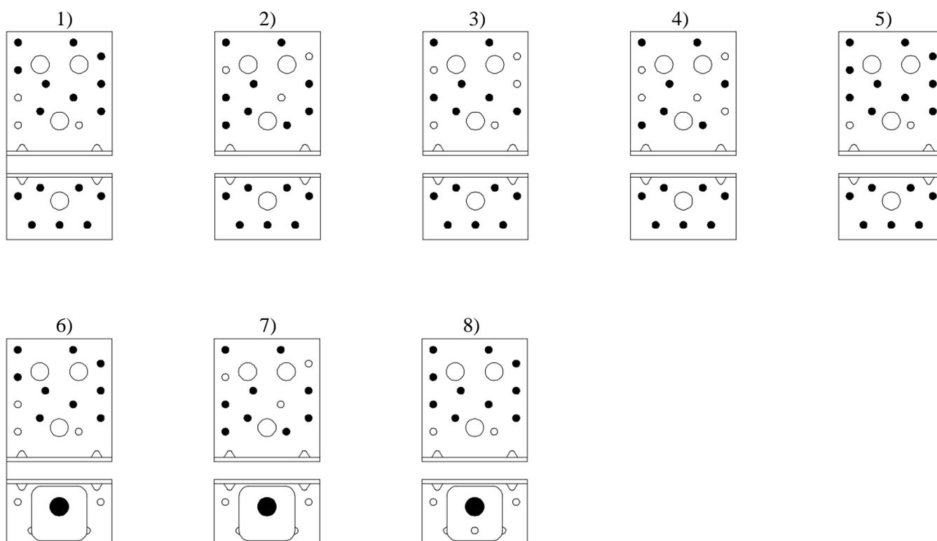
Square washer (US40/40/10G or US40/50/10G) can be replaced by standard washer of the bolts (bolt Ø12 – washer Ø24). In this case the value of  $k_{lat}$  and  $k_{ax}$  must be adapted (see tables below D16-4 and D16-5).
