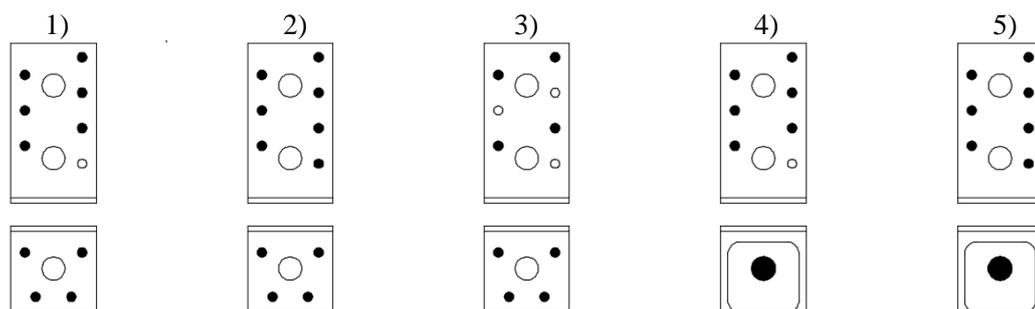
Square washer (US40/40/10G or US40/50/10G) can be replaced by standard washer of the bolts (bolt Ø12 – washer Ø24). In this case the value of  $k_{lat}$  and  $k_{ax}$  must be adapted (see tables below D15-4 and D15-5).
