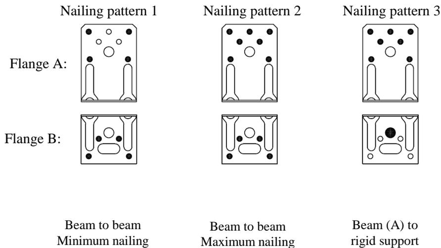
*Table D33-1 Modified characteristic capacity timber beam to timber beam – connector nails.
