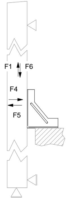
For the nail patterns D to F, it is determined that a vertical load (F6) is always present.
