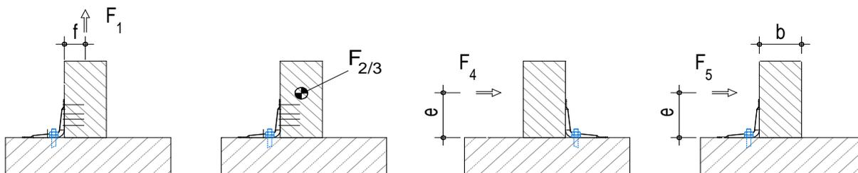
$$R_{i,d} = \frac{R_{i,k} \times k_{mod}}{\gamma_M}$$
