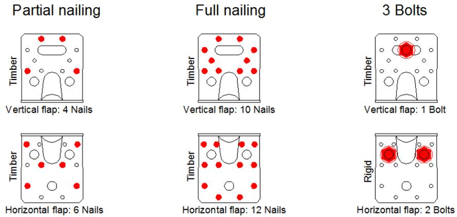
**Table D56-2: Characteristic capacity beam to beam – two Angle Brackets**
