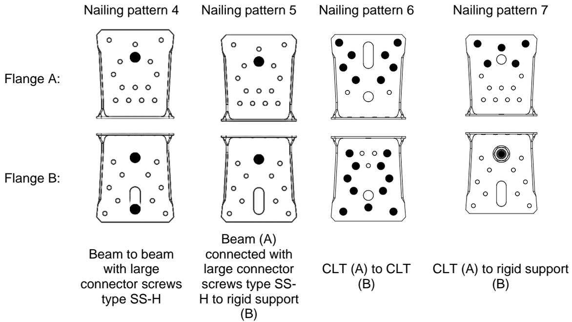
Table D12-1 Modified characteristic capacity timber beam to timber beam – 2 Angle Brackets
