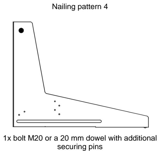
For a downward force, at least the fasteners shown in Nailing pattern 1, 2 and 3 shall be inserted. For an uplift force, the fasteners shown in Nailing pattern 1, 2, 3, and 4 are required.
