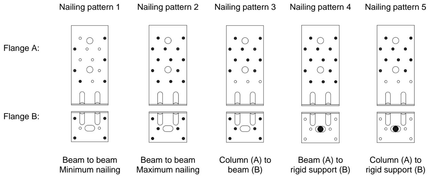
Table D38-1 Modified characteristic capacity timber beam to timber beam – 1 Angle Bracket, Nailing pattern 1
