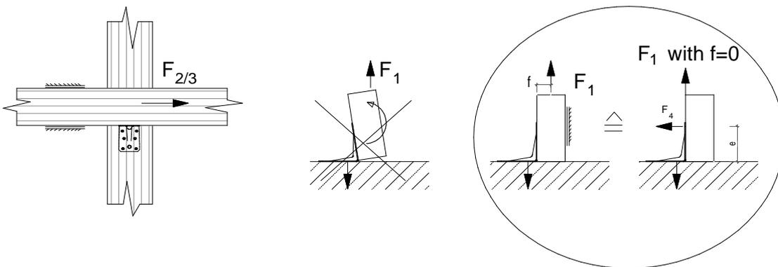
**Table D49-3 Characteristic capacity timber beam to rigid support – 2 Angle Brackets**
