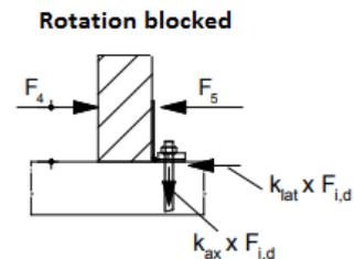
*Table D42-12 Modified characteristic capacity timber column to rigid support – 1 Angle Brackets, Nailing pattern 5*
