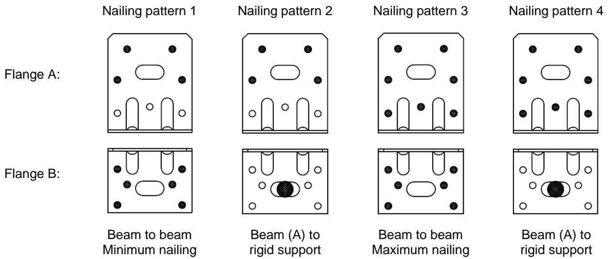
Table D32-1 Modified characteristic capacity timber beam to timber beam - 1 Angle Bracket, Nailing pattern 1
