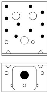
Square washer (US40/40/10G or US40/50/10G) can be replaced by standard washer of the bolts (bolt Ø12 – washer Ø24). In this case, the value of  $k_{lat}$  and  $k_{ax}$  must be adapted (see tables below D16-4 and D16-5).
