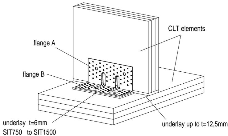
Table D58-3: Characteristic capacity beam to beam – 1 Angle Bracket F<sub>4</sub>
