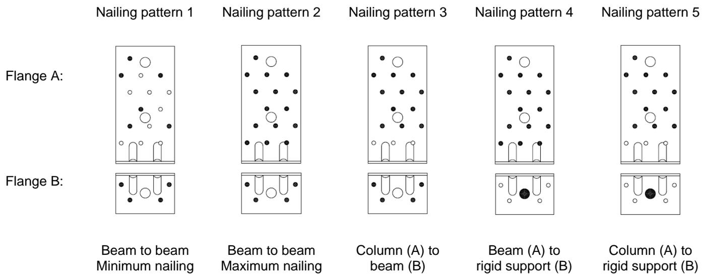
Table D41-1 Modified characteristic capacity timber beam to timber beam – 1 Angle Bracket, Nailing pattern 1
