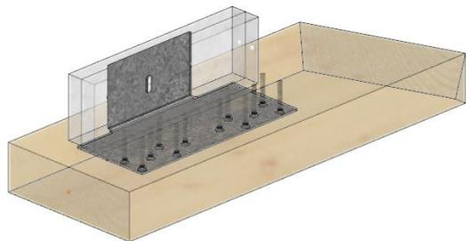
The SC2P-H180 is to fix with 12 CNA4,0x40 on the bottom side of the wall plate.
