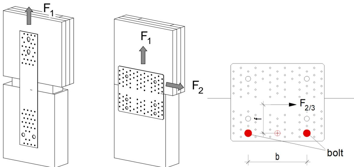
For bolted connection, it's to consider the moment from  $F_2 \times f$  for the bolt group
