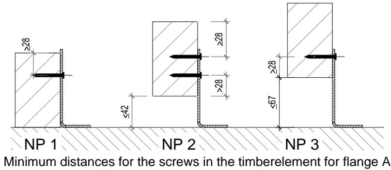
For connection to rigid support has to be check the anchoring as following:
