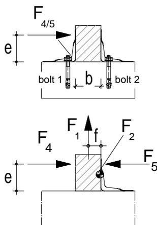
**Table D3-9 Characteristic capacity timber beam to rigid support – 1 Angle Bracket**
