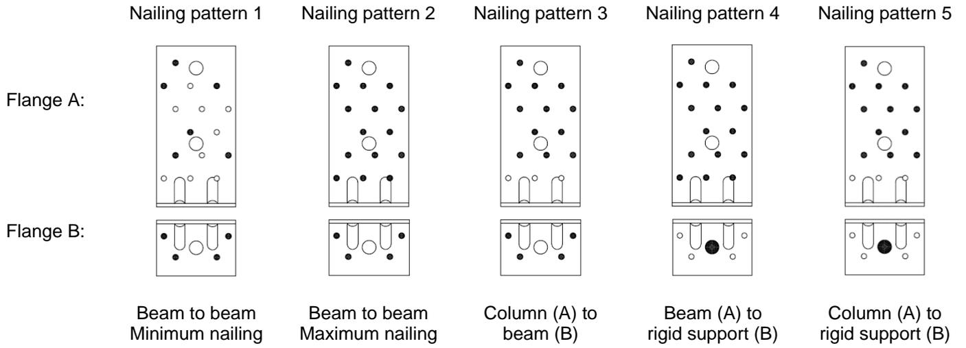
Table D42-1 Modified characteristic capacity timber beam to timber beam – 1 Angle Bracket, Nailing pattern 1
