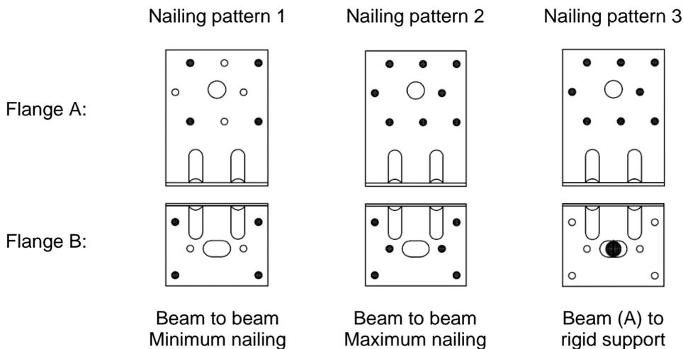
Table D34-1 Modified characteristic capacity timber beam to timber beam – 1 Angle Bracket, Nailing pattern 1
