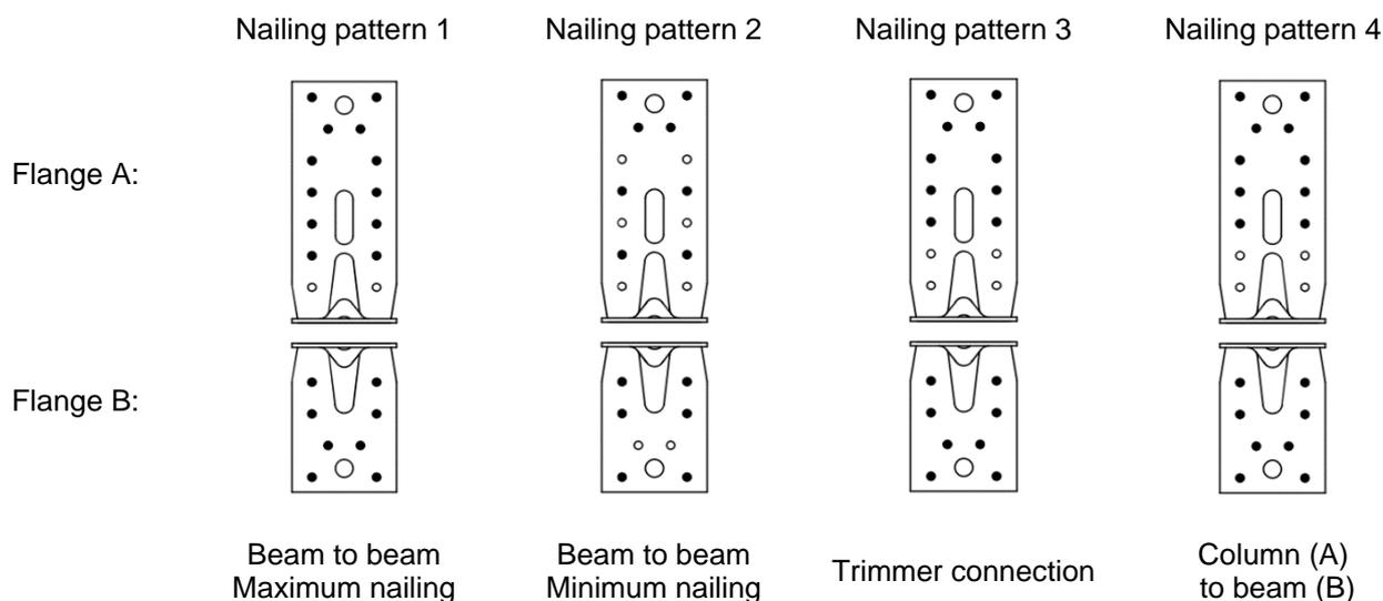
*Table D9-1 Modified characteristic capacity timber beam to timber beam – 2 Angle Brackets*
