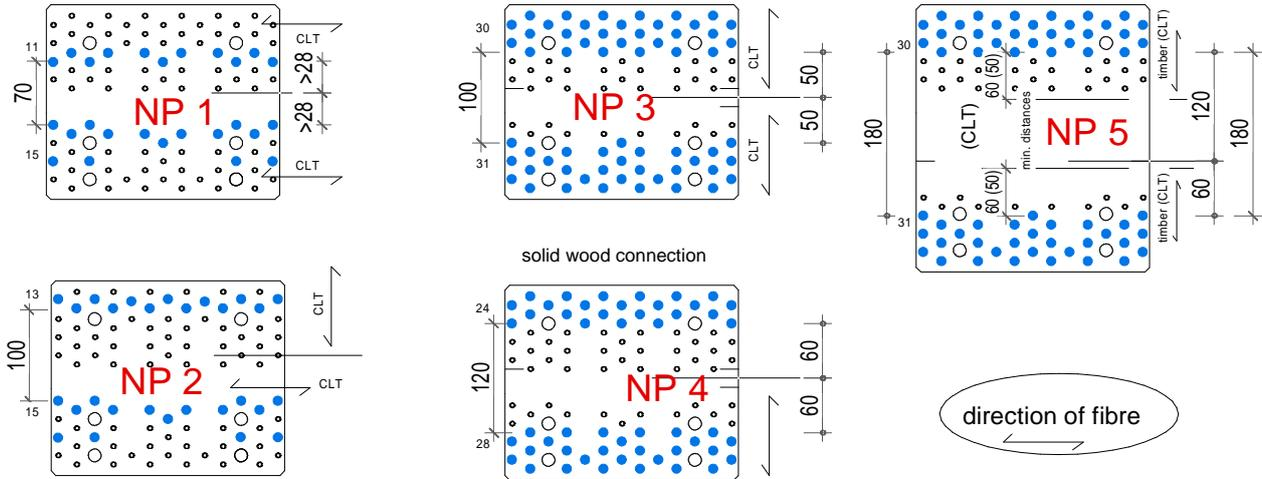
connection timber or CLT to concrete
