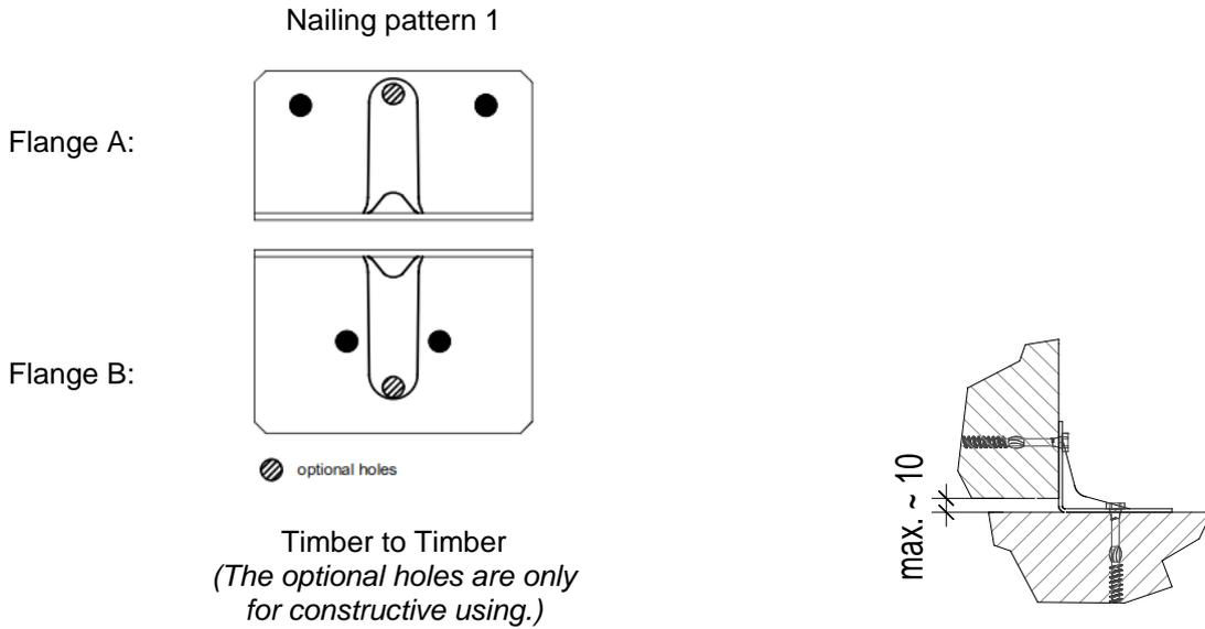
The connected elements shall be free of twisting, so that no rotation occurs.
