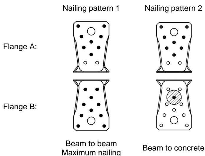
**Table D10-1 Modified characteristic capacity timber beam to timber beam – 2 Angle Brackets**
