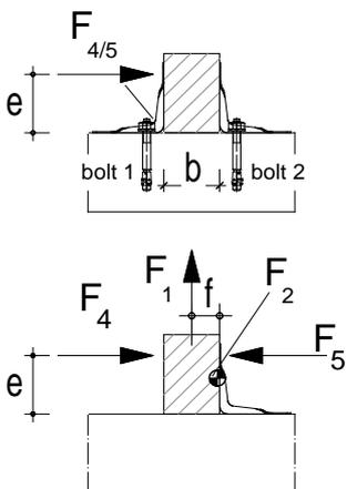
**Table D2-6 Characteristic capacity timber beam to rigid support – 1 Angle Bracket**
