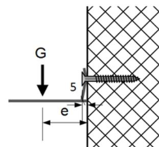
The concrete screw/bolt is subjected to a shear force of  $F_{v,k} = G_k$  and a tension force of  $F_{ax,k} = G_k \cdot e / 30$
