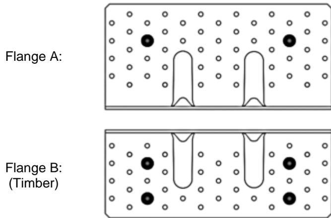
Timber beam (A) to timber beam (B)
