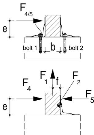
**Table D1-9 Characteristic capacity timber beam to rigid support – 1 Angle Bracket**
