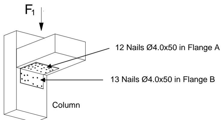
**Table D46-6** Characteristic capacity timber beam to rigid support – 1 Angle Bracket
