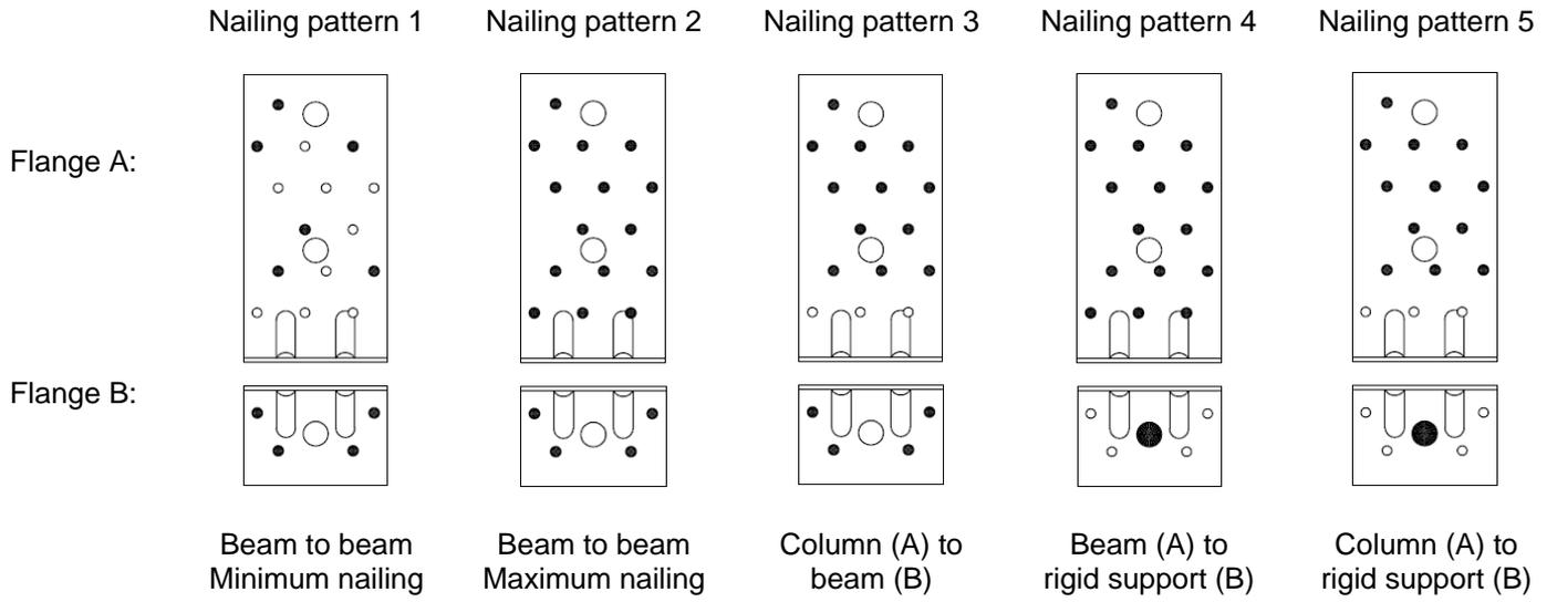
Table D40-1 Modified characteristic capacity timber beam to timber beam – 1 Angle Bracket, Nailing pattern 1
