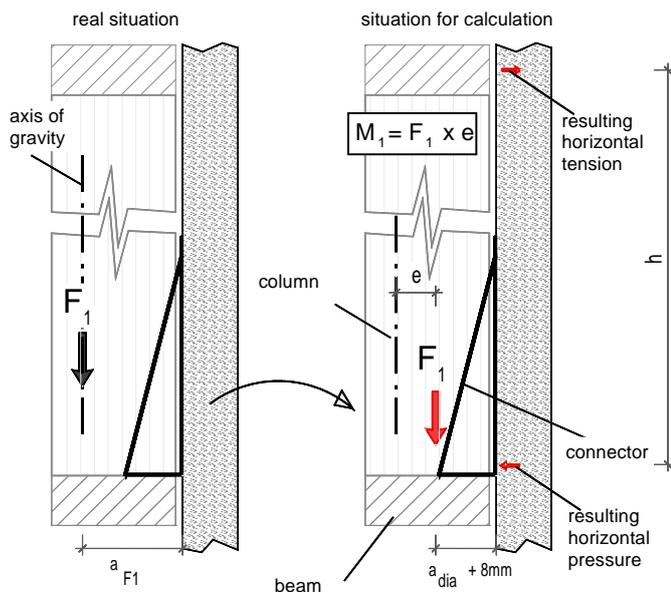
Generally the brackets shall be calculated with a lever arm of  $F_1$  of  $a_{F1} = (a_{dia} + 8mm)$
