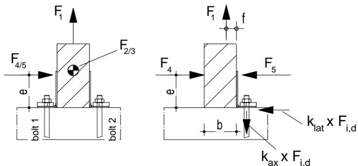
Each bolt shall have a capacity to sustain a lateral force of:  $\geq k_{\text{lat}} \times F_{i,d}$
