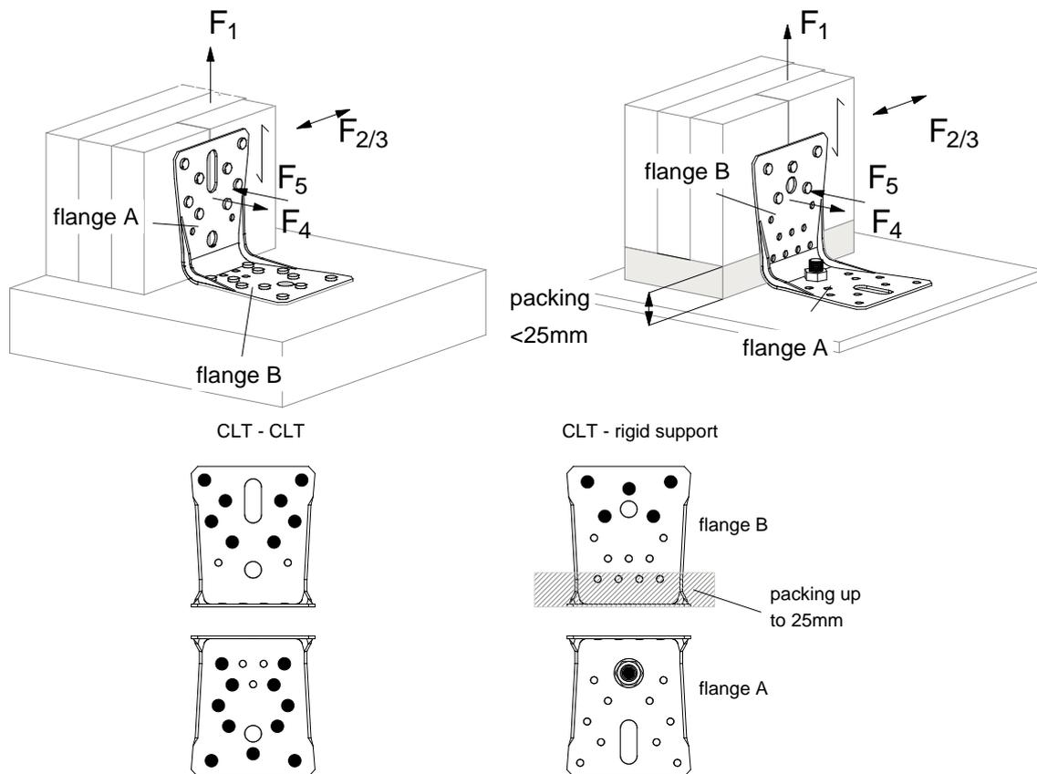
The direction of the outer layer may be also as shown below. (horizontal or vertical)
