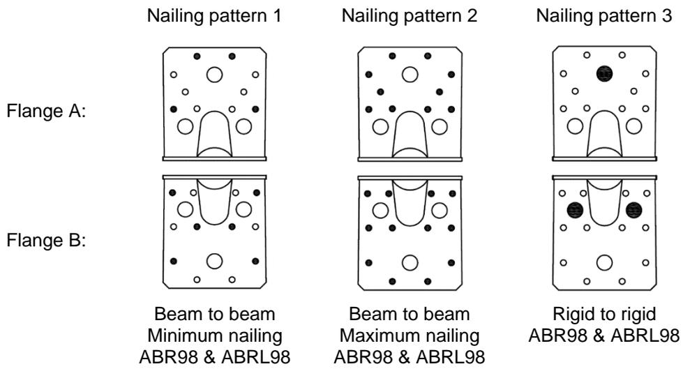
**Table D56-1 Characteristic capacity beam to beam – 2 Angle Brackets**
