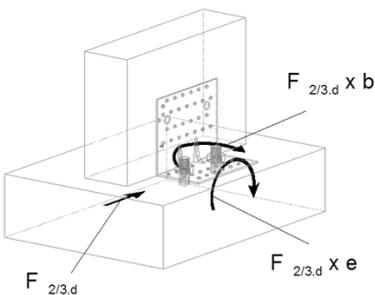
Table D58-7: Characteristic capacity beam to rigid support – 1 Angle Bracket  $F_4$
