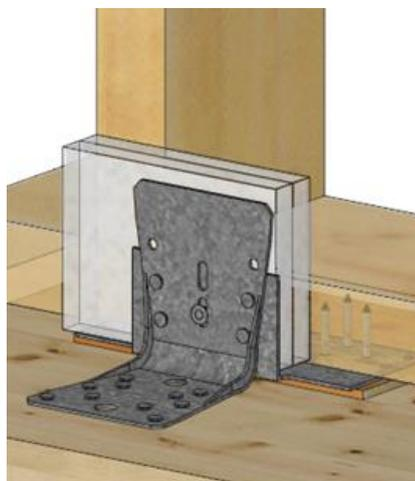
The SC2P-V100 is fixed with the  $\varnothing 6$ mm screw through the oblong holes to the wall element, and with 1 (or 2) bolt(s) to the floor or with CNA4,0x50.
