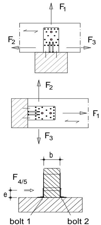
For connection with 2 Angle Brackets it must be checked:
