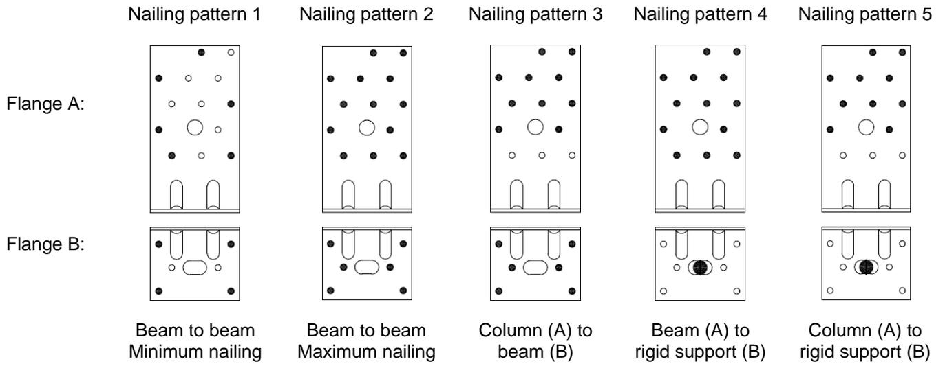
Table D37-1 Modified characteristic capacity timber beam to timber beam – 1 Angle Bracket, Nailing pattern 1
