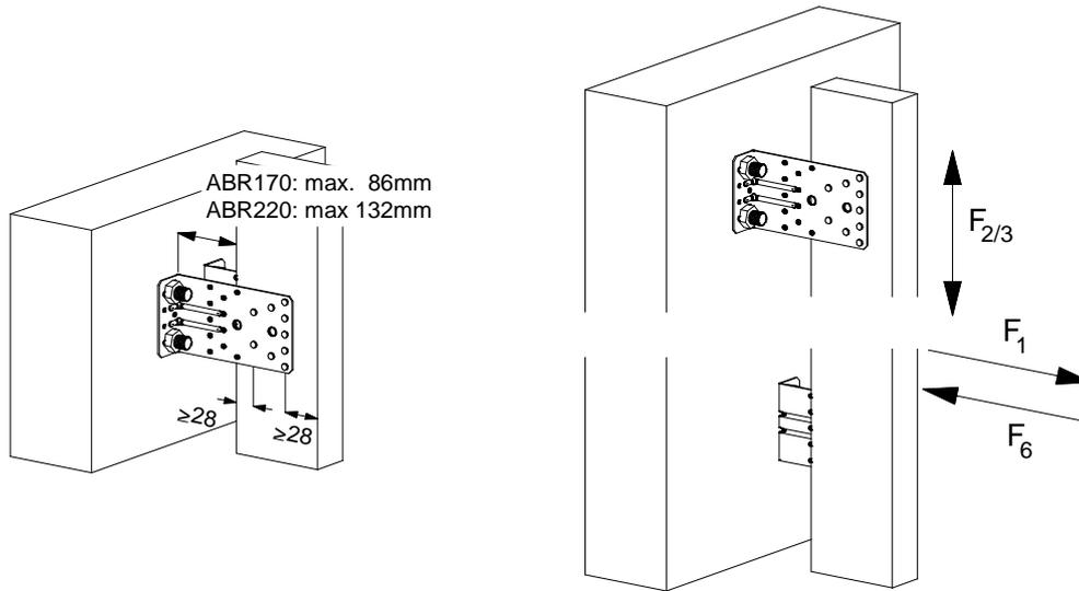
In case of combined force the relevant of the following inequalities shall be fulfilled:
