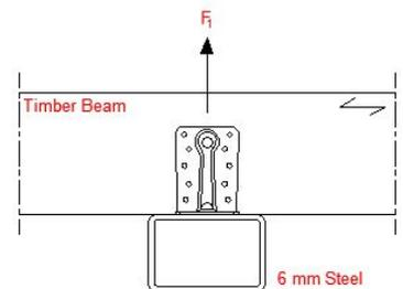
*Table D47-6 Characteristic capacity timber beam to timber column – 1 Angle Bracket*
