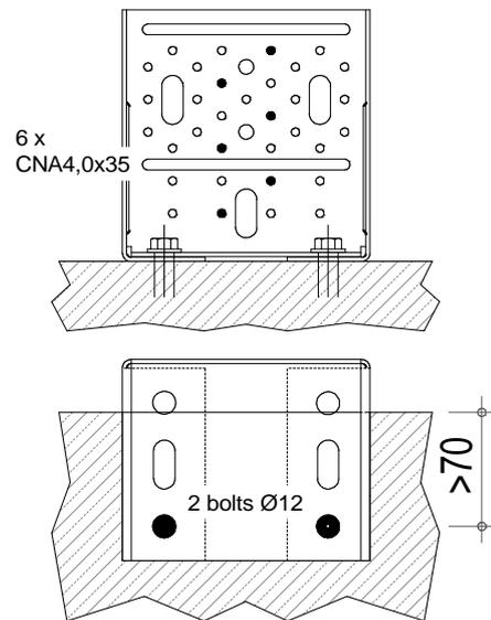
For the nail/bolt pattern A and B, the bolts are positioned with a sufficient distance to any border. The other nail/bolt patterns are for anchorage which has a minimum of 70 mm distance to the border of the concrete.
