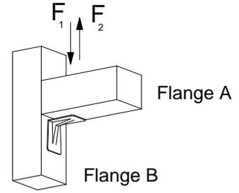
*Table D47-7 Characteristic capacity timber column to timber beam – 2 Angle Bracket*
