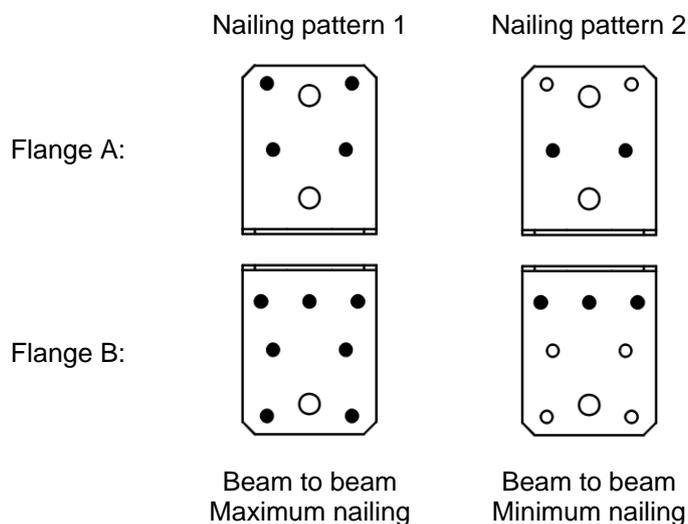
Table D6-1 Modified characteristic capacity timber beam to timber beam – 2 Angle Brackets
