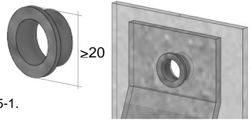
For the distances of the bolts in the beam has to be observe the EN1995-1. The drilling in the beam should be done on site.
