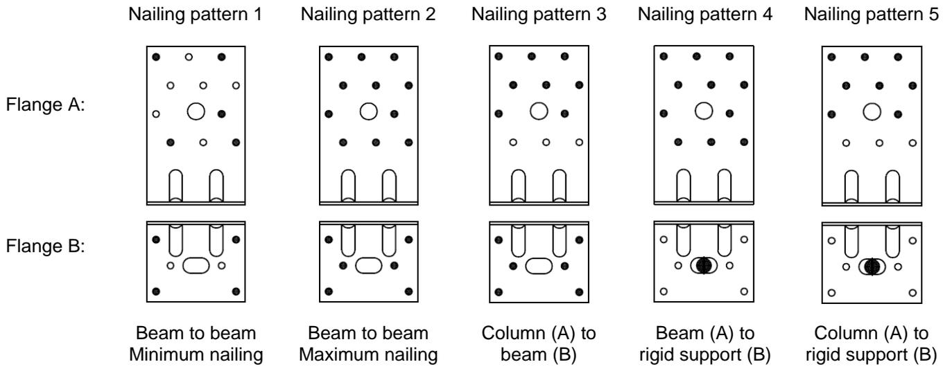
Table D36-1 Modified characteristic capacity timber beam to timber beam – 1 Angle Bracket, Nailing pattern 1
