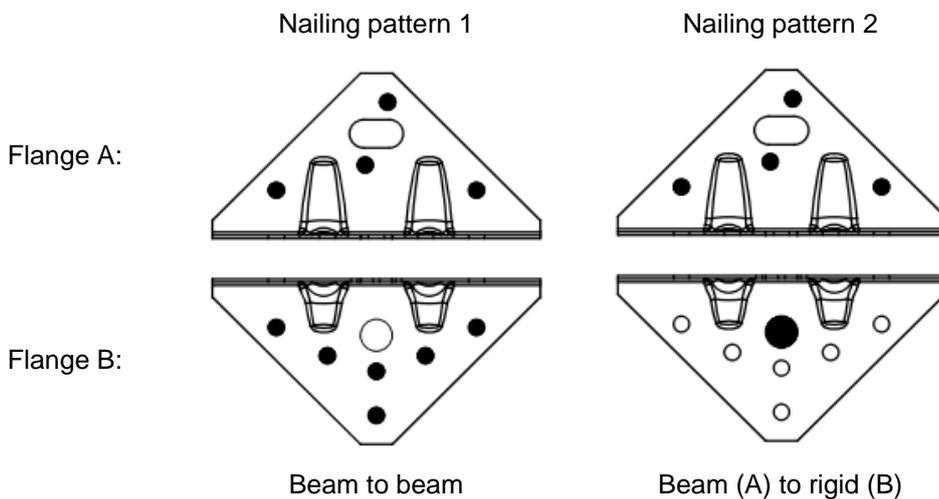
*Table D51-1 Characteristic capacity timber beam to timber beam – 2 Angle Brackets*
